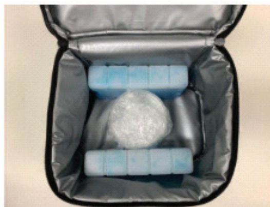
Figure 2. Wrap petri dishes in bubble wrap and pack into a cooler bag with ice bricks.
