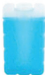
Figure 1. Premium ice bricks are required to keep samples cold (e.g., 4°C) during transport. Please use 3 x 350ml (medium) or 2 x 500ml (large).
