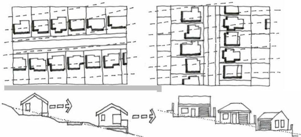
Roads that follow contours (left) minimise cut and fill, the need for unsightly retaining walls, and maximise long distance views. Roads that traverse contours (right) require retaining walls, which impair the streetscape, and increase the potential for overlooking into neighbouring properties.
