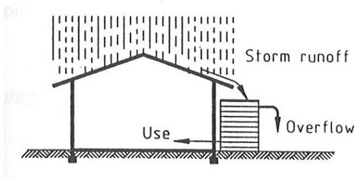
New homes and household extensions of greater than 50m<sup>2</sup> are required to install a rainwater plumbed for internal use which must have a capacity of at least 1,000 kL. Studies have demonstrated that a 3,500 kL tank is able to supply water for indoor use 90% of the time in Mt Barker.
